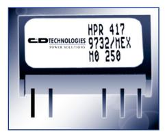
The HPR4XX Series uses advanced circuit design and packaging technology to realize superior reliability and performance. A 170kHz push-pull oscillator is used in the input stage. The HPR4XX Series reduces beat-frequency oscillation problems when used with high frequency isolation amplifiers. Reduced parts count and high efficiency add to the reliability of the HPR4XX Series.
