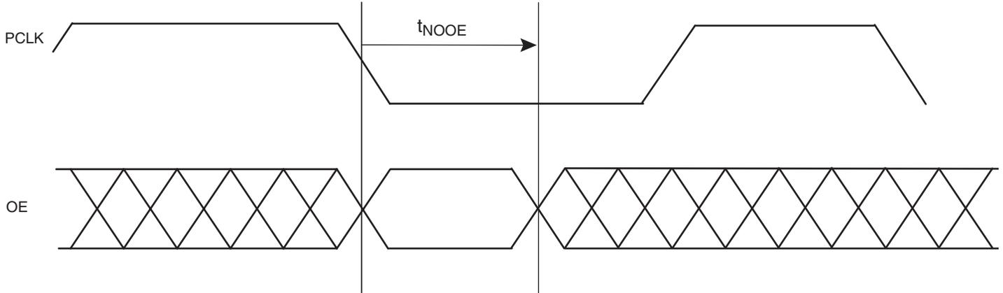
Note: OE must not change during TNOOE after the PCLK falls. This is to ensure that the output drivers of the data are not driving current, so as to reduce the noise level on the power supply.
