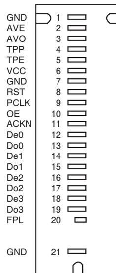
**Table 2-2.** Pin Description for COB with Connector Package: AT77C102B-CB02YV<sup>(1)</sup>
