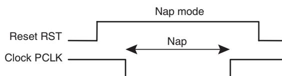
In nap mode, all internal transistors are in shut mode. Only leakage current is drained in the power supply, generally less than the tested value.
