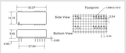
Note: All Pins on a 2.54mm pitch; all pin diameters are 0.50mm; all dimensions in mm.
