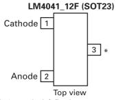
\* Pin 3 must be left floating or connected to pin 2
