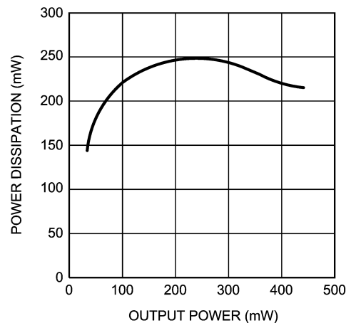
Power Dissipation vs Output Power V_{DD} = 3V, R_L = 8\Omega
