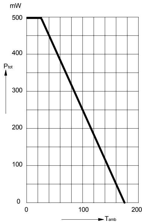
FIG.2 – ADMISSIBLE POWER DISSIPATION VERSUS AMBIENT TEMPERATURE
