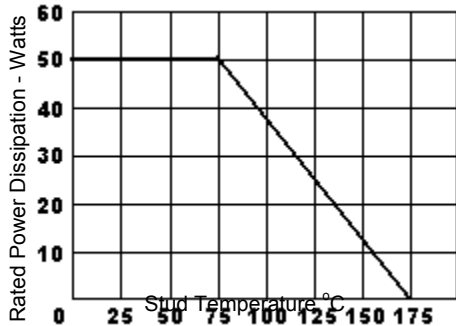
FIGURE 1 Power Derating Curve
