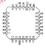
The SN54LS604, SN54LS606, and SN54LS607 are characterized for operation over the full military temperature range of -55 °C to 125 °C; the SN74LS604, SN74LS606, and SN74LS607 are characterized for operation from 0 °C to 70 °C.
