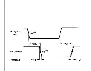
(1) HC:  $V_M$  = 50%;  $V_I$  = GND to  $V_{CC}$ . HCT:  $V_M$  = 1.3 V;  $V_I$  = GND to 3 V.
