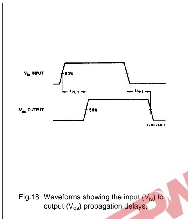
Fig.18 Waveforms showing the input ( $V_{is}$ ) to output ( $V_{os}$ ) propagation delays.
