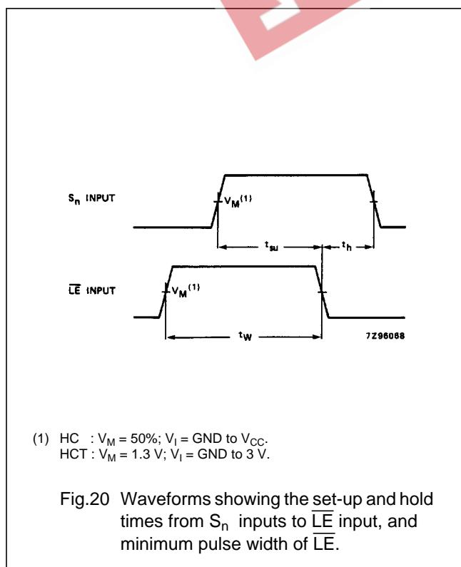
Fig.20 Waveforms showing the set-up and hold times from  $S_n$  inputs to  $\overline{E}$  input, and minimum pulse width of  $\overline{E}$ .
