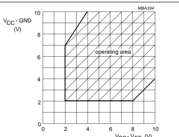
Fig.6 Guaranteed operating area as a function of the supply voltages for 74HC4353.
