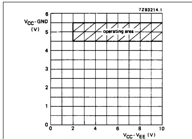
Fig.7 Guaranteed operating area as a function of the supply voltages for 74HCT4353.
