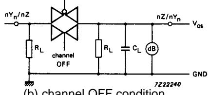
Fig.16 Test circuits for measuring crosstalk between any two switches/multiplexers.
