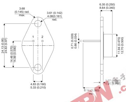
Bipolar NPN Device in a Hermetically sealed TO66 Metal Package.
