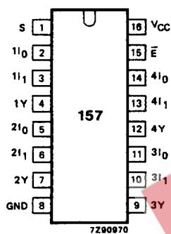
Fig.1 Pin configuration.
