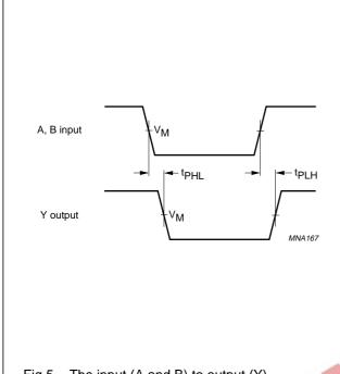
Fig.5 The input (A and B) to output (Y) propagation delays.
