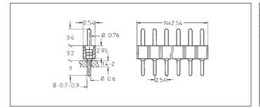
Straight pin connector: solder tail, single row, short pin
