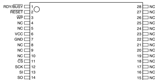
TSOP Top View Type 1
