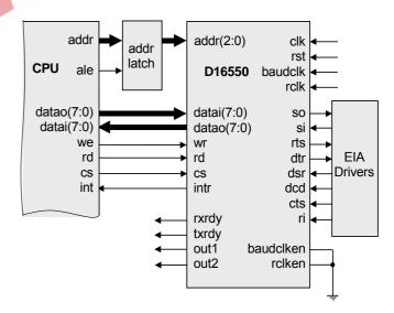
Typical D16550 and processor connection is shown in figure above.
