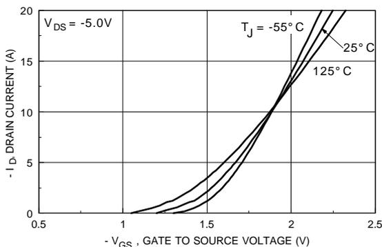
Figure 5. Transfer Characteristics.
