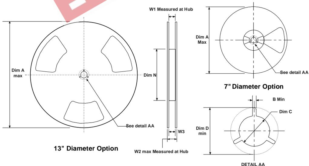
Dimensions are in inches and millimeters
