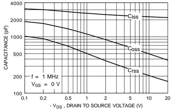
**Figure 8. Capacitance Characteristics.**
