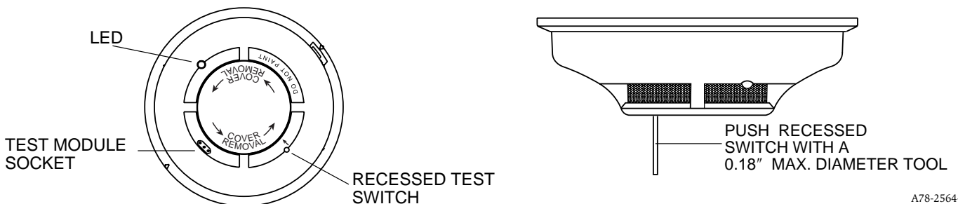
Figure 4. Top and side views showing position of test switch:
