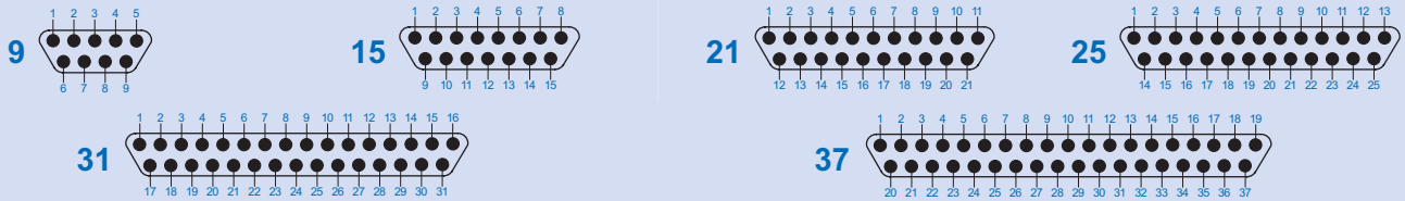
Mating Face View of Pin Connector. Socket connectors have reversed cavity numbers.
