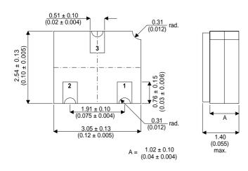
Bipolar NPN Device in a **Hermetically sealed LCC1 Ceramic Surface Mount Package for High Reliability Applications**
