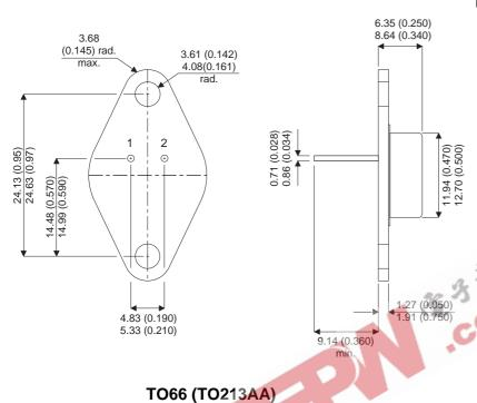
Bipolar NPN Device in a Hermetically sealed TO66 Metal Package.
