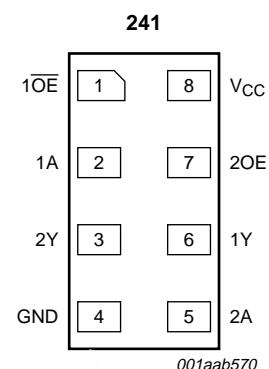
Fig.2 Pin configuration XSON8.
