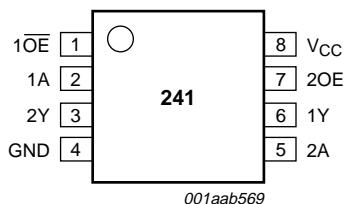
Fig.1 Pin configuration TSSOP8 and VSSOP8.
