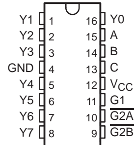
D, N, OR PW PACKAGE (TOP VIEW)
