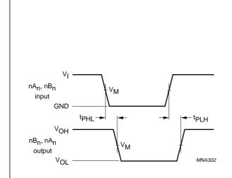
Fig.6 The inputs nA<sub>n</sub>, nB<sub>n</sub> to outputs nB<sub>n</sub>, nA<sub>n</sub> propagation delay times.
