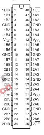
The 74AC16640 is packaged in TI's shrink small-outline package, which provides twice the I/O pin count and functionality of standard small-outline packages in the same printed-circuit-board area.
