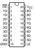
A buffered output-enable  $(\overline{OE})$  input can be used to place the eight outputs in either a normal logic state (high or low) or the high-impedance state. In the high-impedance state, the outputs neither load nor drive the bus lines significantly. The high-impedance state and increased drive provide the capability to drive bus lines without interface or pullup components.
