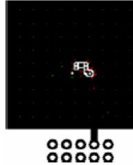
c) 86^\circ\text{C/W} when mounted on a 1\text{in}^2 pad of 2 oz copper.
