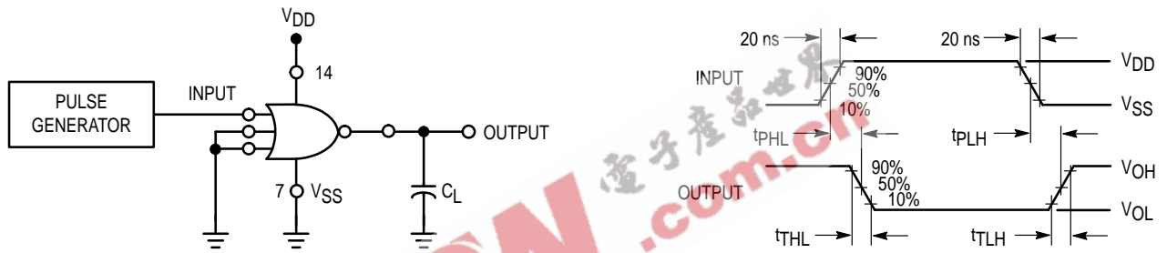
Figure 1. Switching Time Test Circuit and Waveforms
