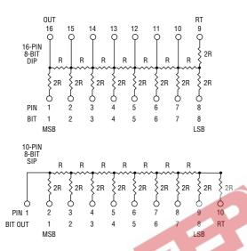
The R/2R Ladder Network is commonly used for Digital to Analog (D/A) conversions and Analog to Digital (A/D) conversion by successive approximations. The bits of the ladder are the points at which input signals are presented to the ladder and the output terminal (OUT) is the point at which the output is
