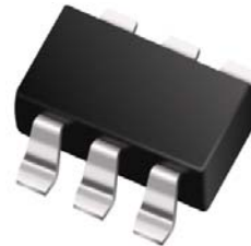
Figure 2. Package Type SC-70
