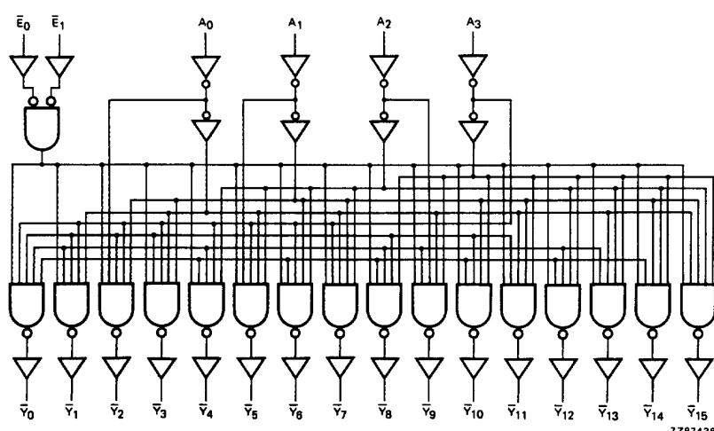
Fig.5 Logic diagram.
