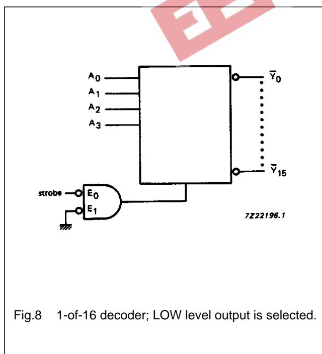
Fig.8 1-of-16 decoder; LOW level output is selected.
