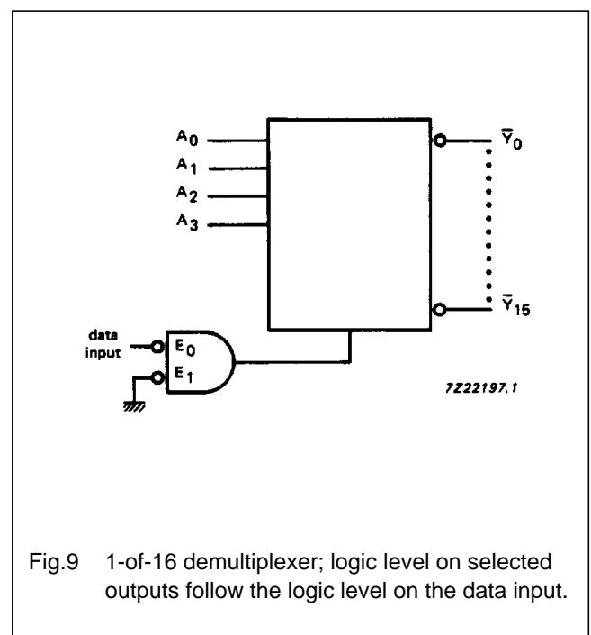
Fig.9 1-of-16 demultiplexer; logic level on selected outputs follow the logic level on the data input.
