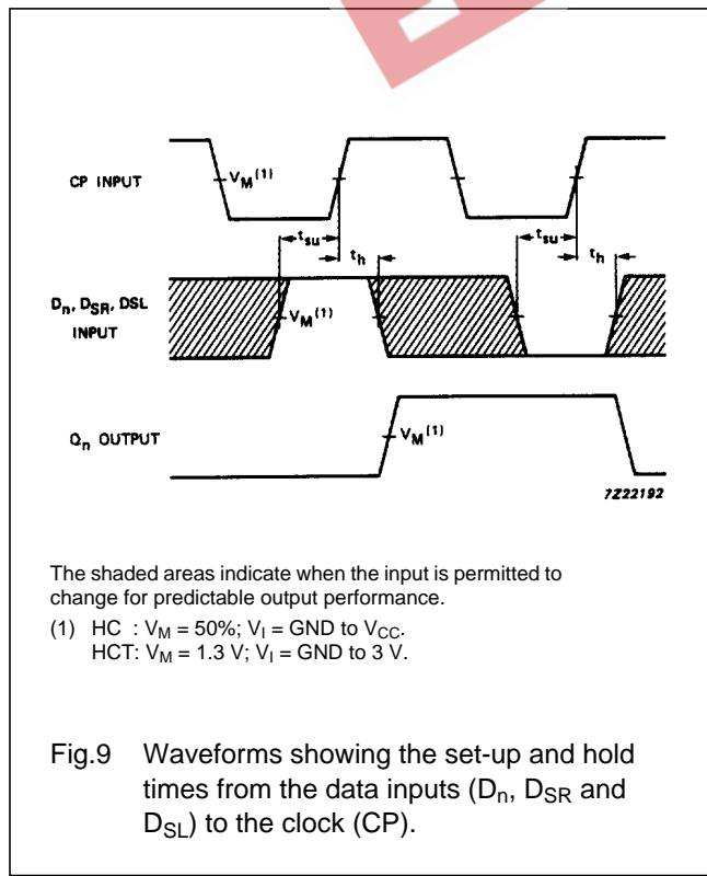
The shaded areas indicate when the input is permitted to change for predictable output performance.
