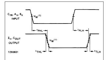
(1) HC :  $V_M$  = 50%;  $V_I$  = GND to  $V_{CC}$ . HCT:  $V_M$  = 1.3 V;  $V_I$  = GND to 3 V.
