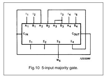
inputs are equally weighted. The outputs  $\Sigma$   $_0,$   $\Sigma_1$  and  $\Sigma$   $_2$  produce a binary number equal to the number inputs (I $_1$  to I $_5$ ) that are HIGH. Figure 10 shows a method of implementing a 5-input majority gate. When three or more inputs (I $_1$  to I $_5$ ) are HIGH, the output M $_5$  is HIGH.
