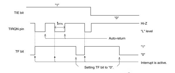
The auto-return time ( $t_{RTN}$ ), shown in the following figure and table, is determined by the source clock frequency set by register 8 in bank 2 bits TD0 and TD1.
