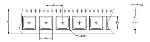
Carrier tape design is defined largely by the component lentgh, width, and thickness
