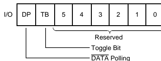
Figure 1. Status Bit Assignment
