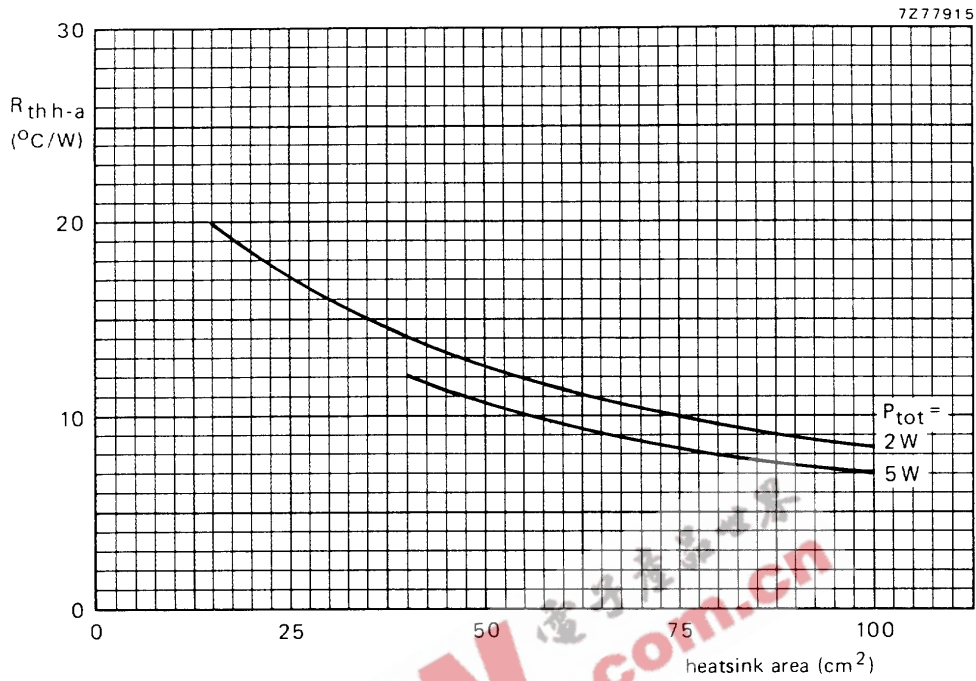
Fig.8 Thermal resistance from heatsink to ambient of a 1,5 mm thick bright aluminium heatsink as a function of the single-sided area of the heatsink with the total power dissipation as a parameter.
