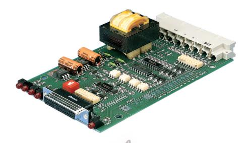
handshaking can be controlled from either end of the communication link. Typical applications involve connecting a host computer to remotely located serial devices such as printers, control equipment, or data acquisition devices distributed throughout an office or factory.
