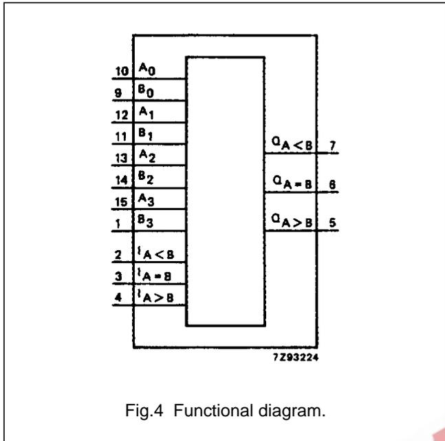
Fig.4 Functional diagram.
