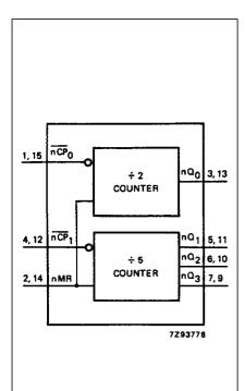
Fig.4 Functional diagram.
