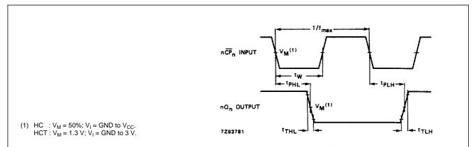
Fig.6 Waveforms showing the clock  $(n\overline{CP}_n)$  to output  $(nQ_n)$  propagation delays, the clock pulse width, the output transition times and the maximum clock frequency.
