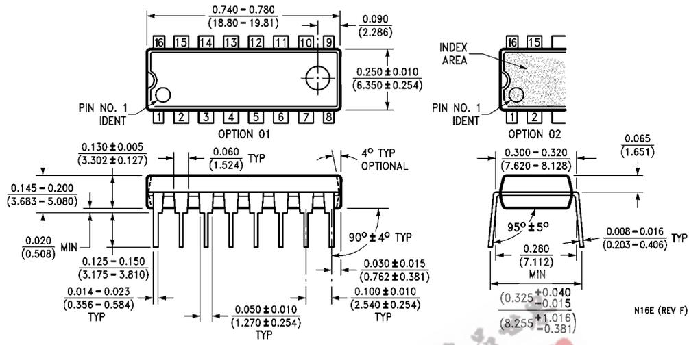
16-Lead Plastic Dual-In-Line Package (PDIP), JEDEC MS-001, 0.300" Wide
