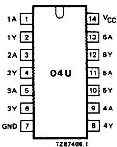
Fig.1 Pin configuration.
