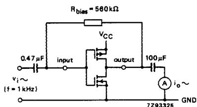
Fig.10 Test set-up for measuring forward transconductance  $g_{fs} = di_o/dv_i$  at  $v_o$  is constant (see also graph Fig.11).
