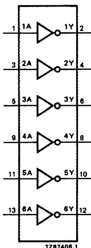
Fig.4 Functional diagram.
