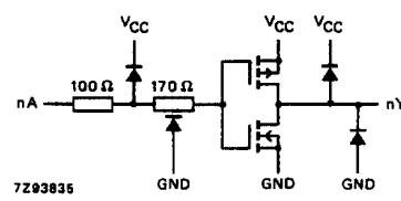
Fig.5 Schematic diagram (one inverter).
