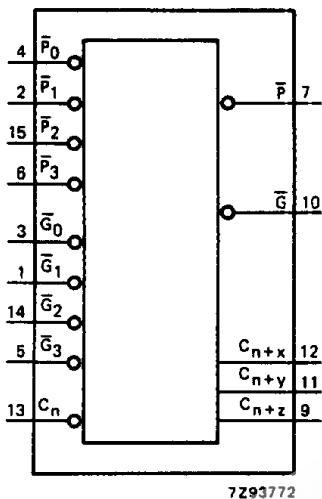
Fig.4 Functional diagram.
