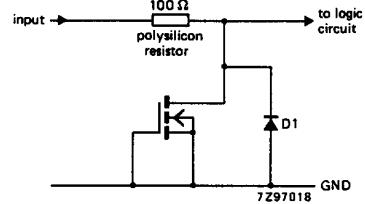
Fig.5 Input protection for HC4050. Single sided thick oxide field effect metal gate transistor as input protection.
