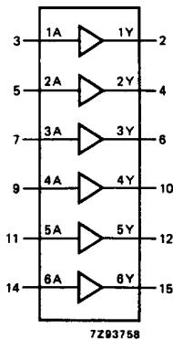
Fig.4 Functional diagram.
