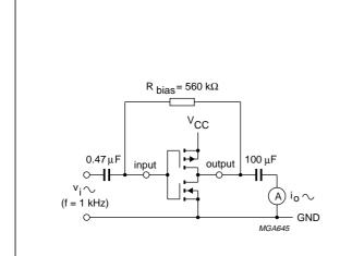
Fig.11 Test set-up for measuring forward transconductance  $g_{fs} = di_o/dv_i$  at  $v_o$  is constant (see Fig.12) and MR = LOW.
