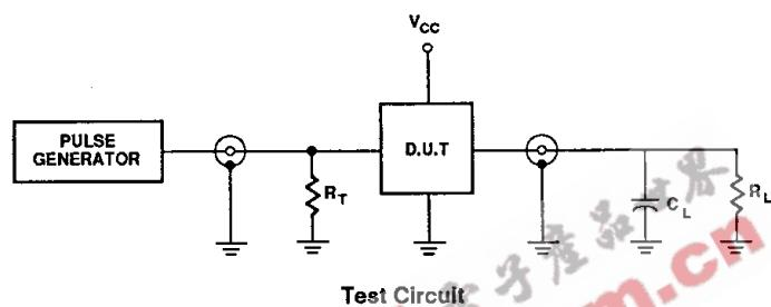
**DEFINITIONS** $C_L$  = Load capacitance, 50pF; includes jig
