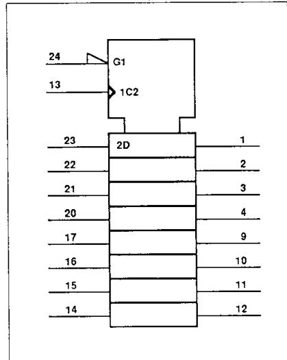
**Octal D-type flip-flop with enable****74AC/ACT11377****PIN DESCRIPTION**
