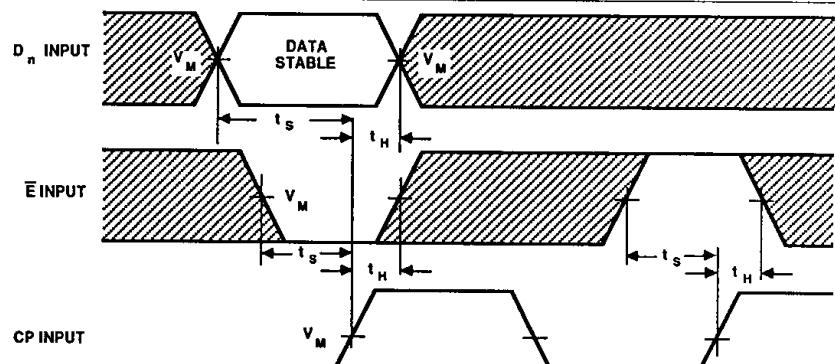
Waveform 3. Waveforms Showing the Data Set-up and Hold Times for the Input ( $D_n$ ) and Parallel Enable Input ( $\bar{E}$ )
