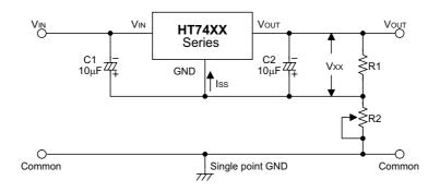
$$V_{\text{OUT}} \ = \ V_{\text{XX}} \ (\ 1 + \frac{\text{R2}}{\text{R1}}\ ) \ + \ I_{\text{SS}} \ \text{R2}$$
