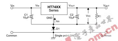
$$V_{OUT} = V_{XX} + V_{D}$$
