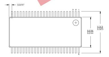
DIMENSIONS IN INCHES  $\underline{\text{MIN.}}_{\text{MAX.}}$
