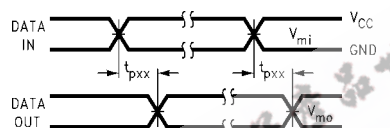
FIGURE 2. Waveform for Inverting and Non-inverting Functions
