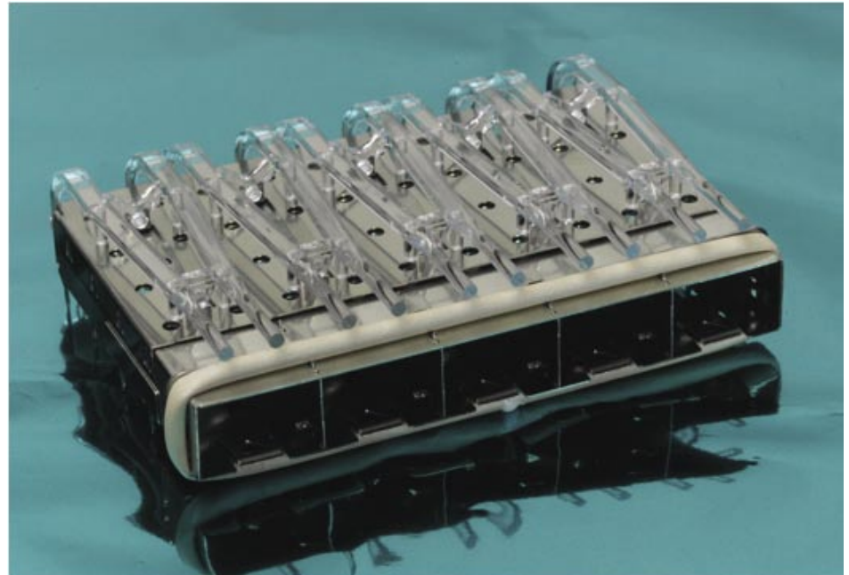
Lightpipe cover mounted on 1-by-5 SFP cage
